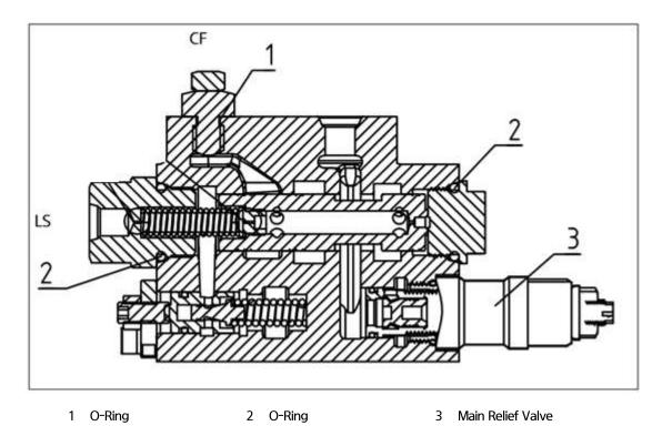
The priority valve is integrated into the main valve. The valve is affected by the LS signal on the steering device to ensure that sufficient oil is supplied to the steering circuit. The valve maintains a constant steering force and speed to resist changes in the pump hydraulic oil supply flow, and first supplies hydraulic oil to the steering circuit.
